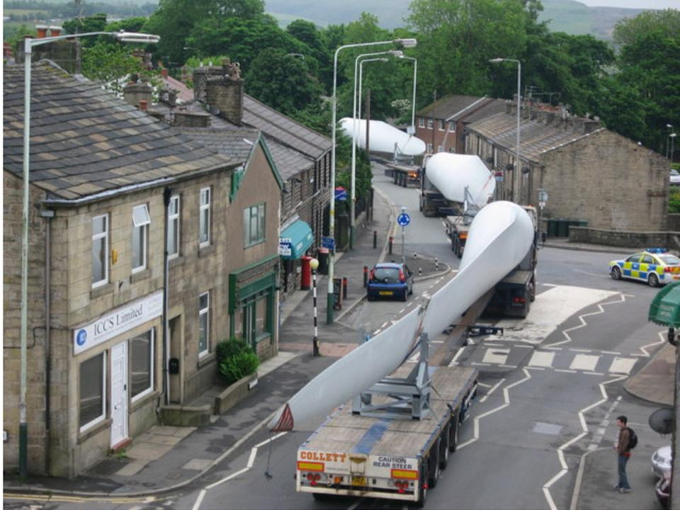
Figure 1: **A convoy of wind turbine blades passing through the village of Edenfield, England.**
