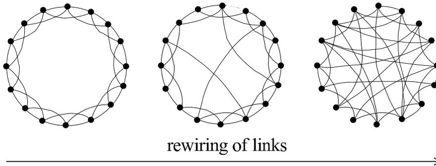
Left hand side: one-dimensional lattice with connections between all vertex pairs by two or fewer lattice spaces away. A Small World is created by randomly rewiring edges.
