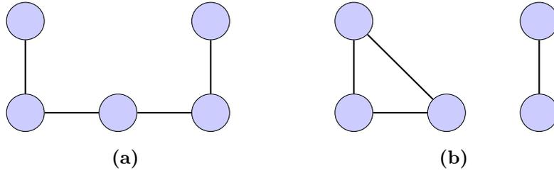
**Figure 4:** Two networks with equal degree distribution but different topology.
