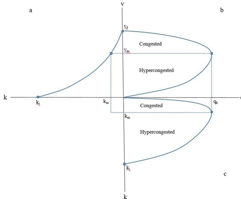
Figure 1: The Fundamental diagram of traffic flow.
