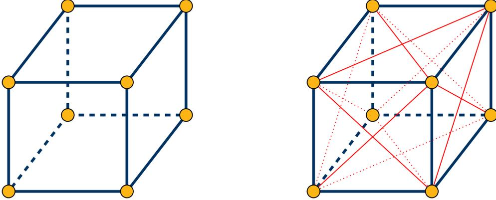
Figure 1: three-dimensional hypercube (left) and extended hypercube (right).
