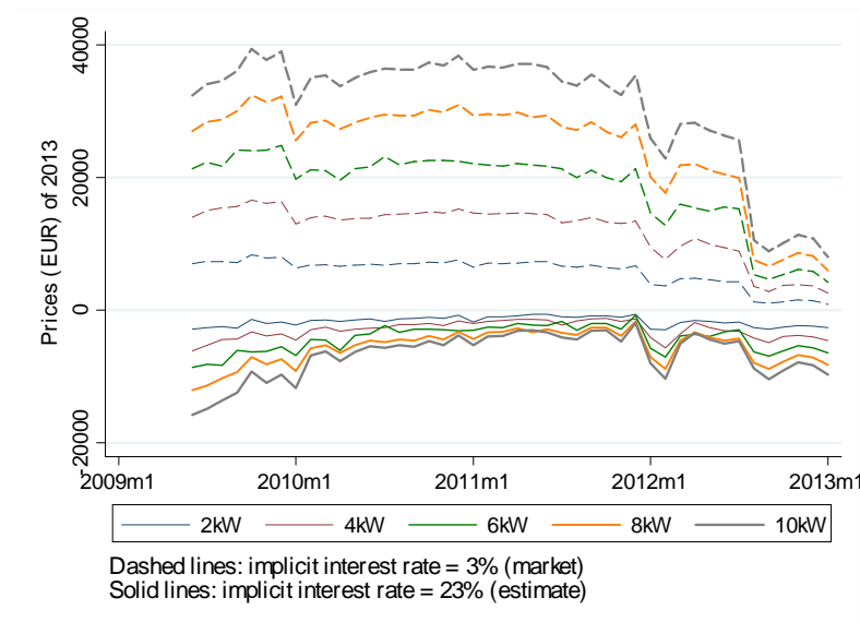
Figure 5: NPV of PVs during 2006-2012 at real, yearly interest rates: market rate and estimate of implicit rate
